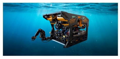
Utilizing underwater Remote Operated Vehicles, commonly known as ROVs, is a safe and cost-effective way to efficiently inspect and assess underwater infrastructure and assets that are not easily accessible by other means. Areas that are prone to limited visibility and potentially tight spaces are ideal for ROVs as these specialized underwater vehicles use high resolution optical and sonar sensors and dynamic positioning equipment to enhance visual acuity and operational maneuverability.
